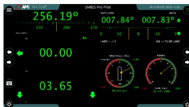
Vessel Movement with Comparator, SMIDS Heading, Bow Fore and Aft Speed, Wind and Rudder Data.
