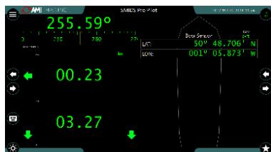
Vessel GNSS Compass, SMIDS Heading, Bow Fore and Aft Speed, and Bow Latitude and Longitude.
