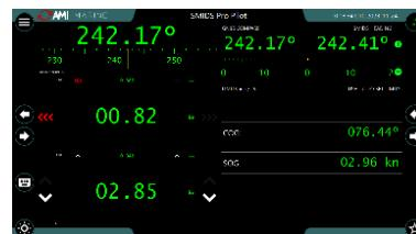
Vessel GNSS Compass, SMIDS Heading, Bow Fore and Aft Speed, Course Over Ground (COG) and Speed Over Ground (SOG).
